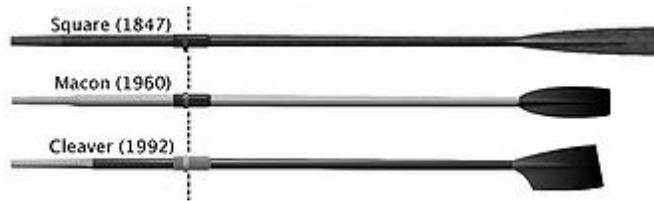
Oars are adjustable. The most common adjustment is at the ‘collar’ that determines how much of the oar is inside or outside the ‘oarlock’ that holds the oar to the boat on the ‘rigger’. Each oar (whether it is a sweep or sculling oar) is designed to be a port or starboard one. Both the asymmetric hatchet blade and collar determine which side the oar fits on.
